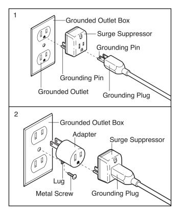
The green-colored rigid ear, lug, or the like extending from the adapter must be connected to a permanent ground such as a properly grounded outlet box cover. The adapter must be held in place by a metal screw. **Some 2-pole receptacle outlet box covers are not grounded. Contact a qualified electrician to determine if the outlet box cover is grounded before using an adapter.**
